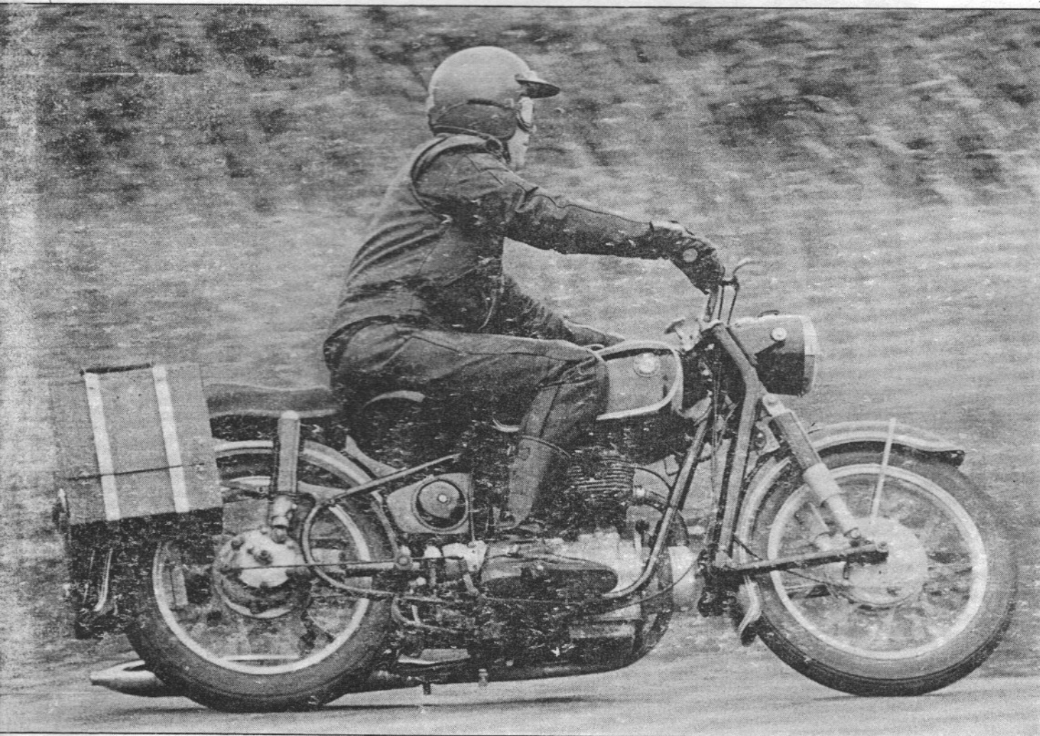
R25/3's plungers have no hydraulic damping: they gave a choppy ride
